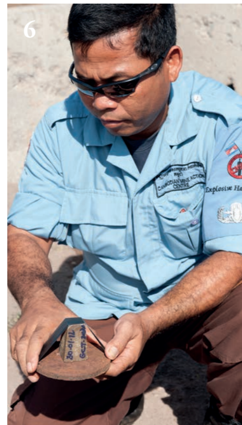
Explosive harvesting 1. The munitions are cut in half to reveal the explosives. 2 & 3. The explosives are steamed out of the shell casing. 4. The explosive is melted and poured into silicone moulds to set. 5. The charges are turned out of the moulds to dry in the sun and are marked with batch number and manufacture date. 6. A sample charge is placed on a steel plate to test the strength of the batch. 7. The steel plate reveals this batch is powerful.
