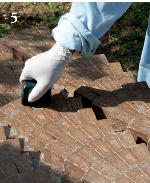
Explosive harvesting 1. The munitions are cut in half to reveal the explosives. 2 & 3. The explosives are steamed out of the shell casing. 4. The explosive is melted and poured into silicone moulds to set. 5. The charges are turned out of the moulds to dry in the sun and are marked with batch number and manufacture date. 6. A sample charge is placed on a steel plate to test the strength of the batch. 7. The steel plate reveals this batch is powerful.
